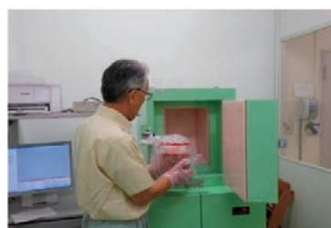
2. Setting a sample to \gamma -ray detector
